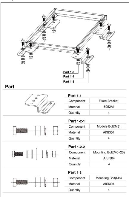
Attached the PV module to the mounting foot using M8 screw/bolt supplied in the pack. Be carful of the bolt, flat washer, spring wash and nut sequences. Find suitable holes on the panel frame and fasten the mounting foot on it.
