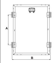
\*Drill holes in the mounting surface by the length of A and B measured from the panel before installation. Mount the panel together with the holes.
